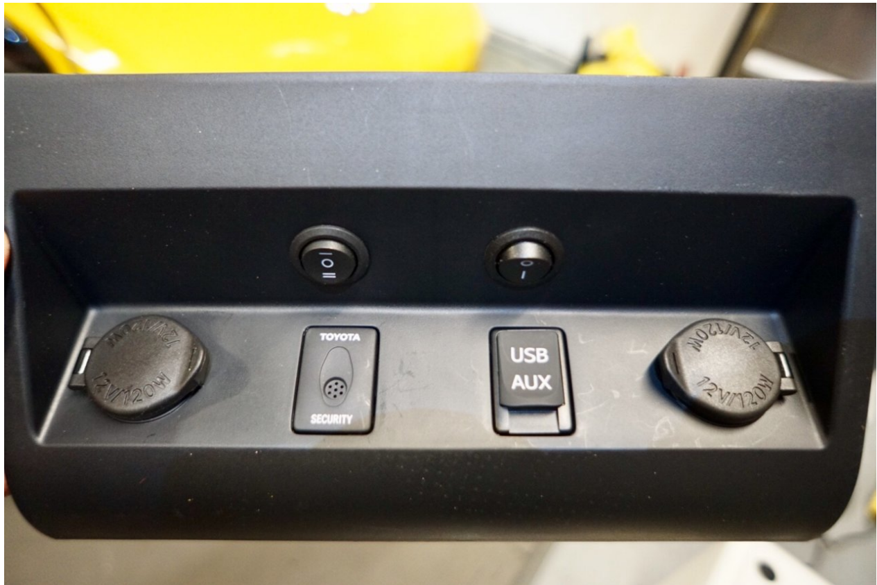
Figure 3: Alternate switch location for 1794, Platinum and some Limited models.
